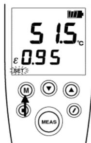
6. Press the **▼** or the **▲** key to change the  $\epsilon$  value until the temperature becomes the value obtained in (3). The  $\epsilon$  value at this time is emissivity of the object to be measured.
